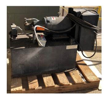
Hydraulic pump with 3 phase 10 HP, Baldor electric motor Frame 215TC, RPM 1720
