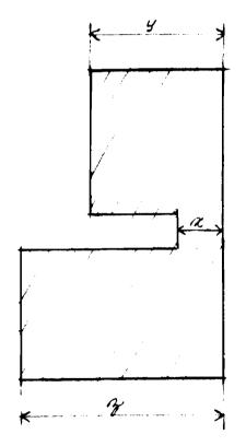
THIS BUILDING IS CONSIDERED AS TWO UNITS, BECAUSE NO IS LESS THAN 3/4 OF B
