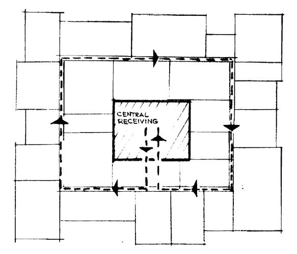
LAY OUT CENTRAL RECEIVING TO SCALE, SURROUNDED BY ALL OTHER SECTIONS, ARRANGED SO AS TO HAVE A TRUCK ROUTE OF MINIMUM LENGTH SERVING ALL SECTIONS.
